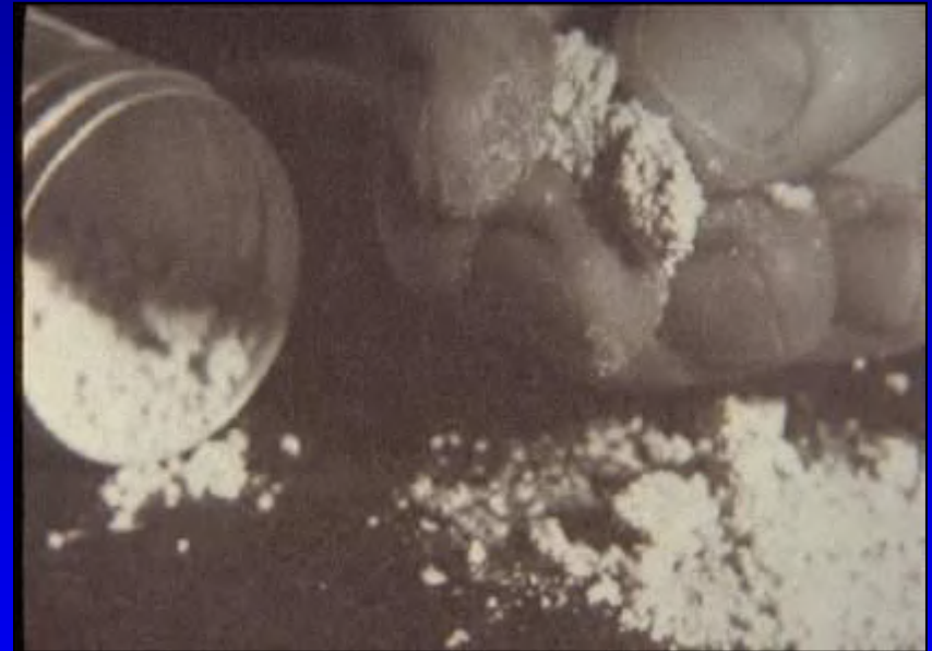
Photo of friable asbestos
