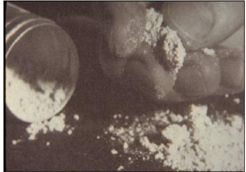
Photo of friable asbestos
