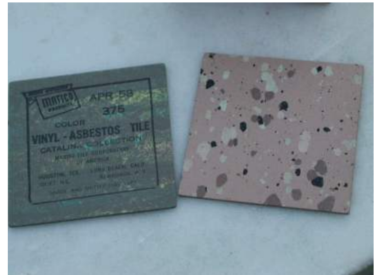
Vinyl asbestos flooring
